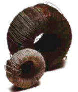
A coil that uses a ferrite core
